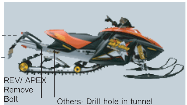
Target Area for mounting the front of the X-Rack to the snowmobile tunnel.
